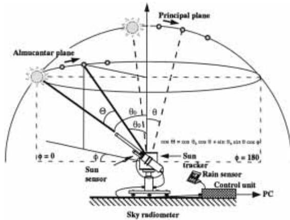
Fig. 2. Geometry of the ground-based sky radiometer system. The sky radiometer includes a sun- and sky-scanning spectral radiometer, a sun sensor, a sun tracker, a control unit, a rain sensor, and a personal computer. Diffuse solar radiation is measured by two different scanning methods depending on the solar zenith angle,  $\theta$ . The scattering angle  $\Theta$  is related to  $\theta_0$ , and to observation angle  $\theta$  and  $\phi$ . See detail in text.
